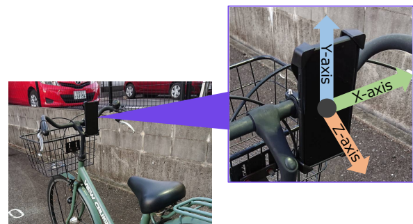
Figure 6: Smartphone attached and acceleration axis
