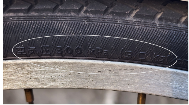
Figure 2: Maximum proper pressure indicated on the side of the tire
