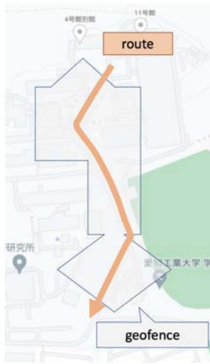
Figure 9: Verification of geofencing operation
