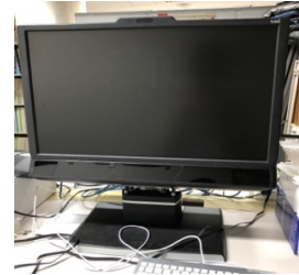
Figure 2 Measurement equipment (Tobii Pro Tx-300)
