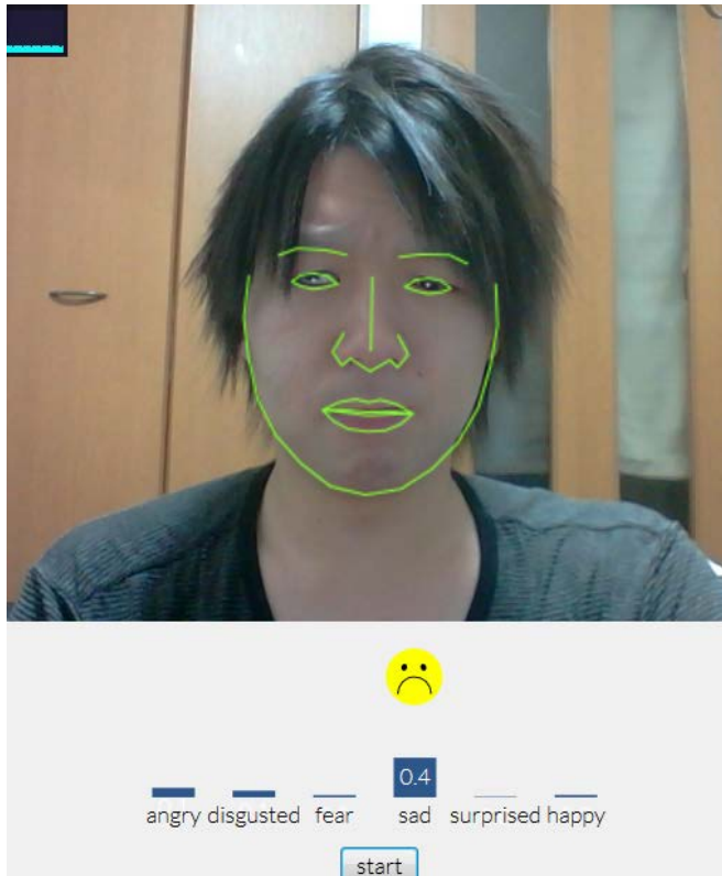
Figure 3: The detection of each emotion by facial expression image in real time
