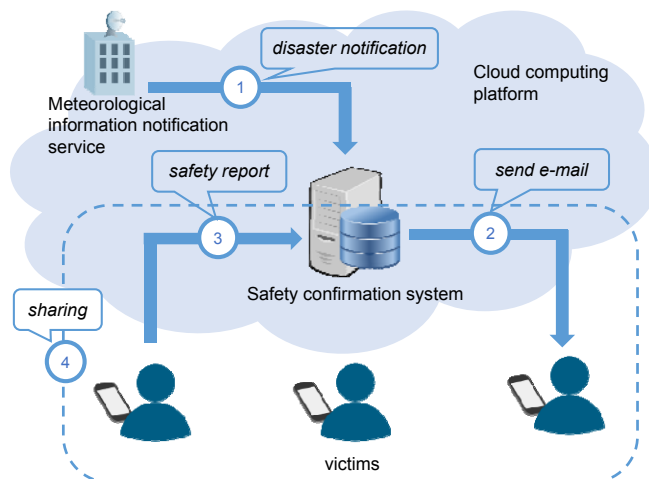
Figure 1: Flow of the safety confirmation system
