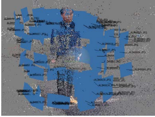
Figure 9: Camera position and point in 3D view
