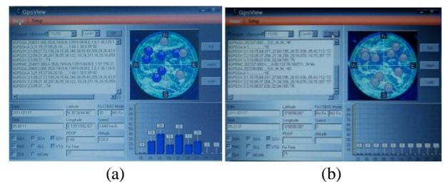
Figure 23: GPS signal conditions (a) Outside of a tunnel, (b) Inside of a tunnel
