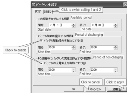
Figure 1: Peak shift setting utility released by Fujitsu Limited.
