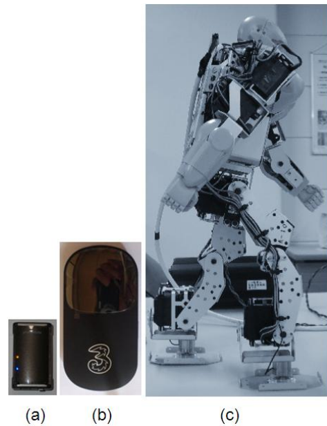
Figure 6: Parts of the agent device. (a) GPS; (b) Mobile Wi-Fi Router, (c) Agent Device [Type of a Smart Robot]
