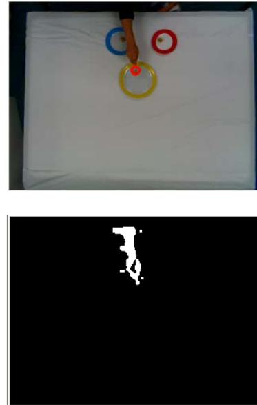
Figure 6: Hand recognition from the ceiling.
